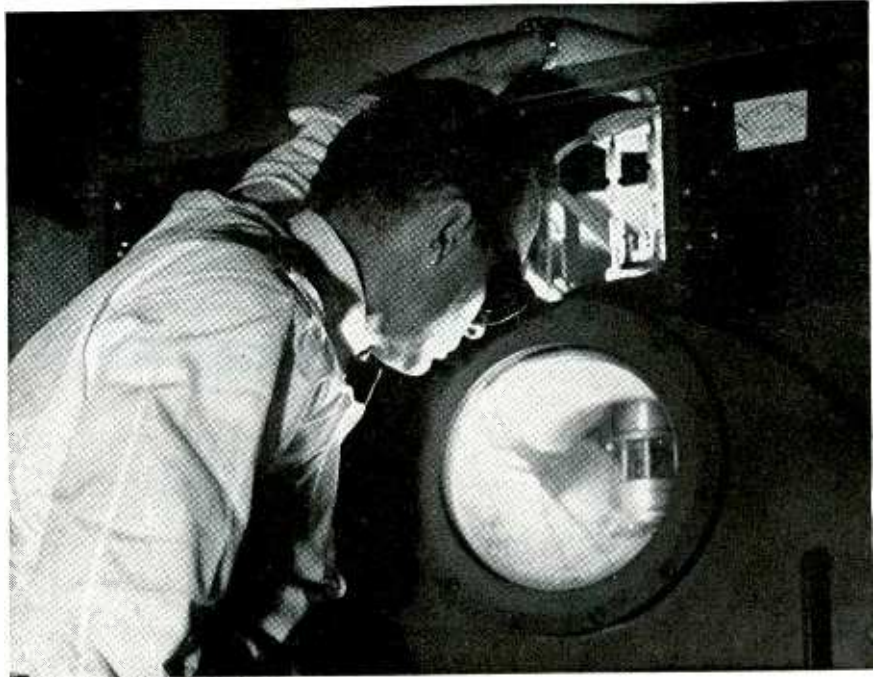
C.B. Sibley, senior development engineer at the National Research Corp. equipment division, adjusts electron beam gun to change focus during operation.
