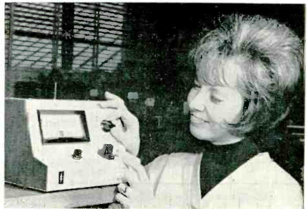
Engineering-laboratory test set for measuring unijunction transistor's characteristics. This instrument whose circuitry contains unijunction transistors, measures seven characteristics including intrinsic standoff ratio and interbase resistance. It is manufactured by the Syracuse Electronics Corp.
