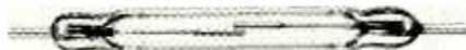
We dynamically set the air gap for each switch (shown here 2X actual size).
