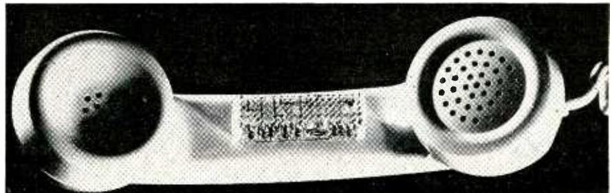
Ministac perched on a telephone receiver. Five of these components stacks are packaged in a Danish transceiver that weighs only two pounds.
